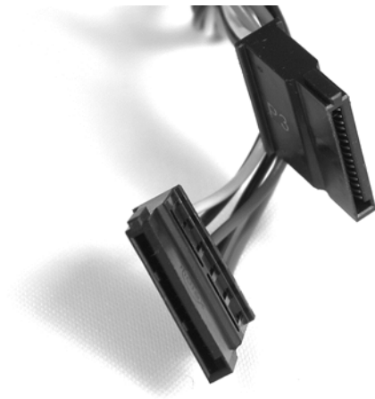
Exhibit 1-4: A serial ATA (SATA) power connector
